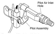
Figure 31 - Pilot Inlet Air Hole
